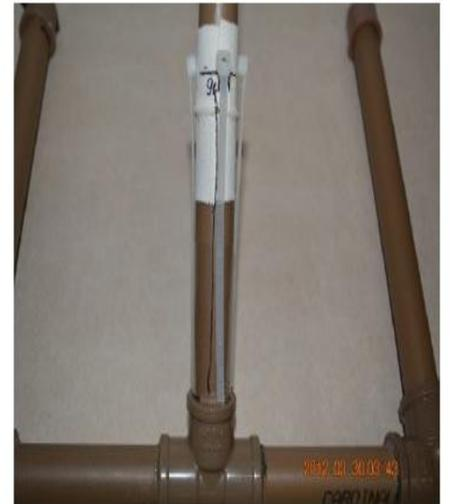
Fig. 15. Base com as 4 abraçadeiras de nylon.
