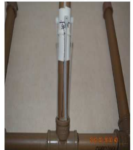
Fig. 15. Base com as 4 abraçadeiras de nylon.
