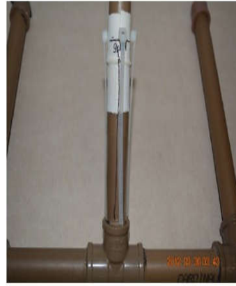
Fig. 15. Base com as 4 abraçadeiras de nylon.
