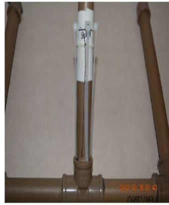
Fig. 15. Base com as 4 abraçadeiras de nylon.
